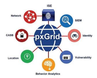
From such intel, ISE can issue a change of authorization (CoA), essentially immediately revoking access to the network and placing the endpoint in a different state (quarantine or offline). A holistic approach to security always has an enforcement mechanism and, from a Cisco technology perspective, ISE is the enforcer.
