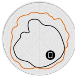
Figure 6. R770 5GHz Elevation Antenna Patterns
