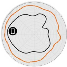
Figure 5. R770 2.4GHz Elevation Antenna Patterns
