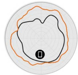
Figure 7. R770 6GHz Elevation Antenna Patterns
